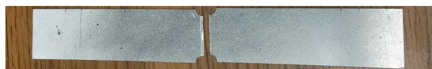
Sample 1 with Speckle Pattern after Failure
