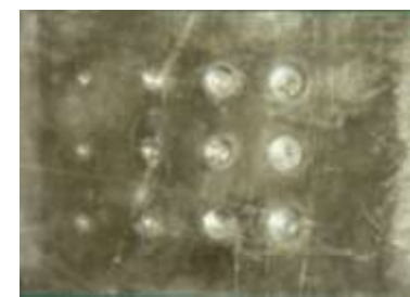
Aluminum 7075 sample with blind hole
